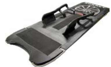
The skeleton sleds are manufactured from stainless and high-strength steels with a thickness of between three and eight millimeters. They consist of cowling, a frame, and two runners. Photo: German institute for the research and development of sports equipment (FES)
