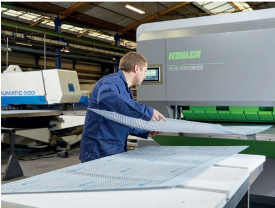
BriMetal uses a KOHLER Peak Performer for leveling. Sheets with a width up to 1600 mm and a thickness up to 17 mm can be leveled.
