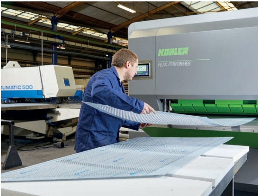
BriMetal uses a KOHLER Peak Performer for leveling. Sheets with a width up to 1600 mm and a thickness up to 17 mm can be leveled.
