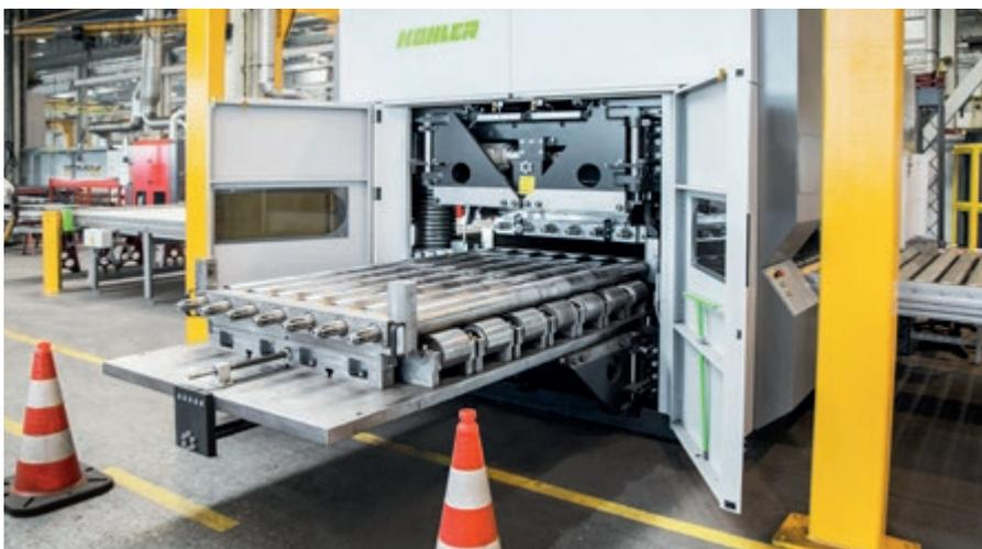
The Peak Performer’s advanced cleaning system enables the leveling rollers and supporting rollers to be fully moved out of the machine, by means of electric motor, for quick, easy cleaning. .
