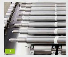
Patented reversible leveling rollers
