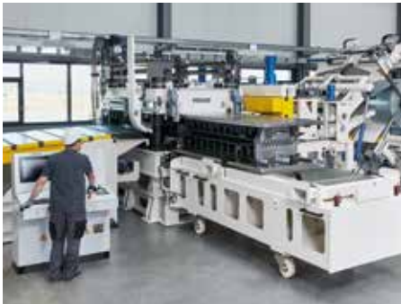
— Interchangeable levelling roller cassette expands the range of strip thicknesses that can be processed
