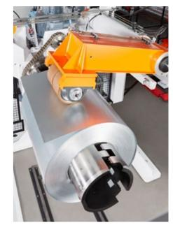
Double decoiler with two expansion ranges without additional expansion elements
