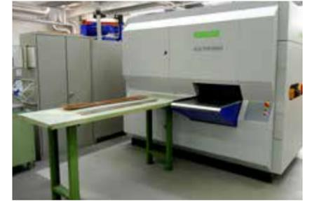
— The compact and neatly enclosed Peak Performer 50P.600 part levelling machine, viewed from the outlet side. The levelled precious metal strips are deposited on the table.
