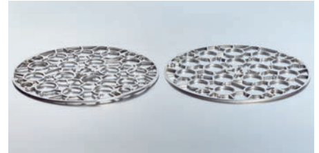
Increased precision and quality: parts of a water treatment system from Xylem. Left: Before leveling. Right: After leveling
