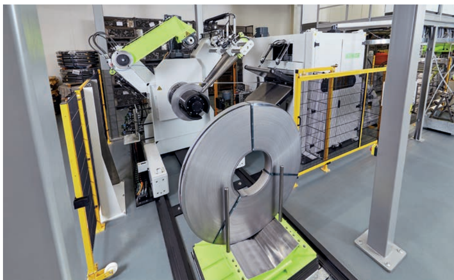
Blickle processes several thousand tons of steel and steel materials every year in its own production facilities. In order to meet future requirements, the company recently invested in a modern and efficient strip leveling line from KOHLER Maschinenbau GmbH.
