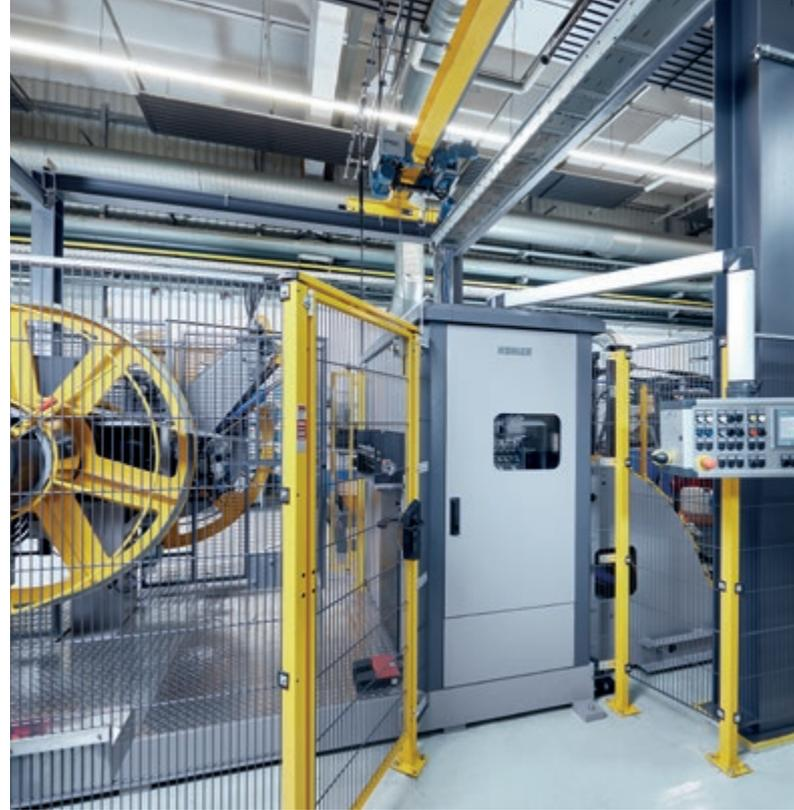
Freiberger EuroMetall uses stamping and edge rimming to produce their coin blanks. The preliminary work is performed by a KOHLER strip feeding line comprising (from left to right) a double decoiler, strip leveling machine and strip transfer to high speed punching machine.
