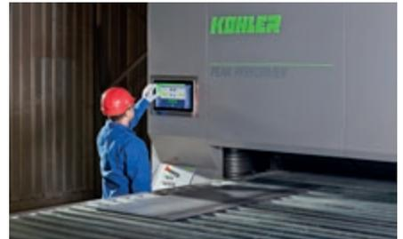
The touch display and intuitive user interface means operators can set up the part leveling machine in just a few steps.
