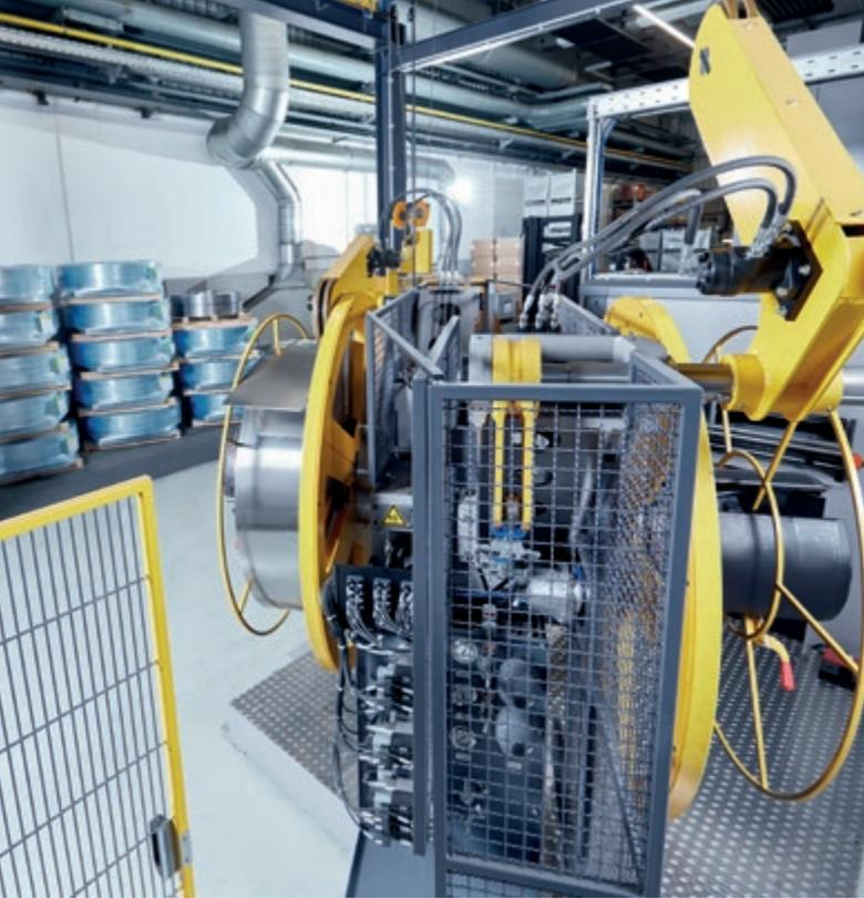
KOHLER double decoiler, type 5000.2 H, for the loading of two coils, up to 5,000 kg each in weight, strip widths of up to 500 mm and strip thicknesses of up to 3 mm. The coils are fixed to the mandrels using a hydraulic sliding wedge system with automatic retensioning system.
