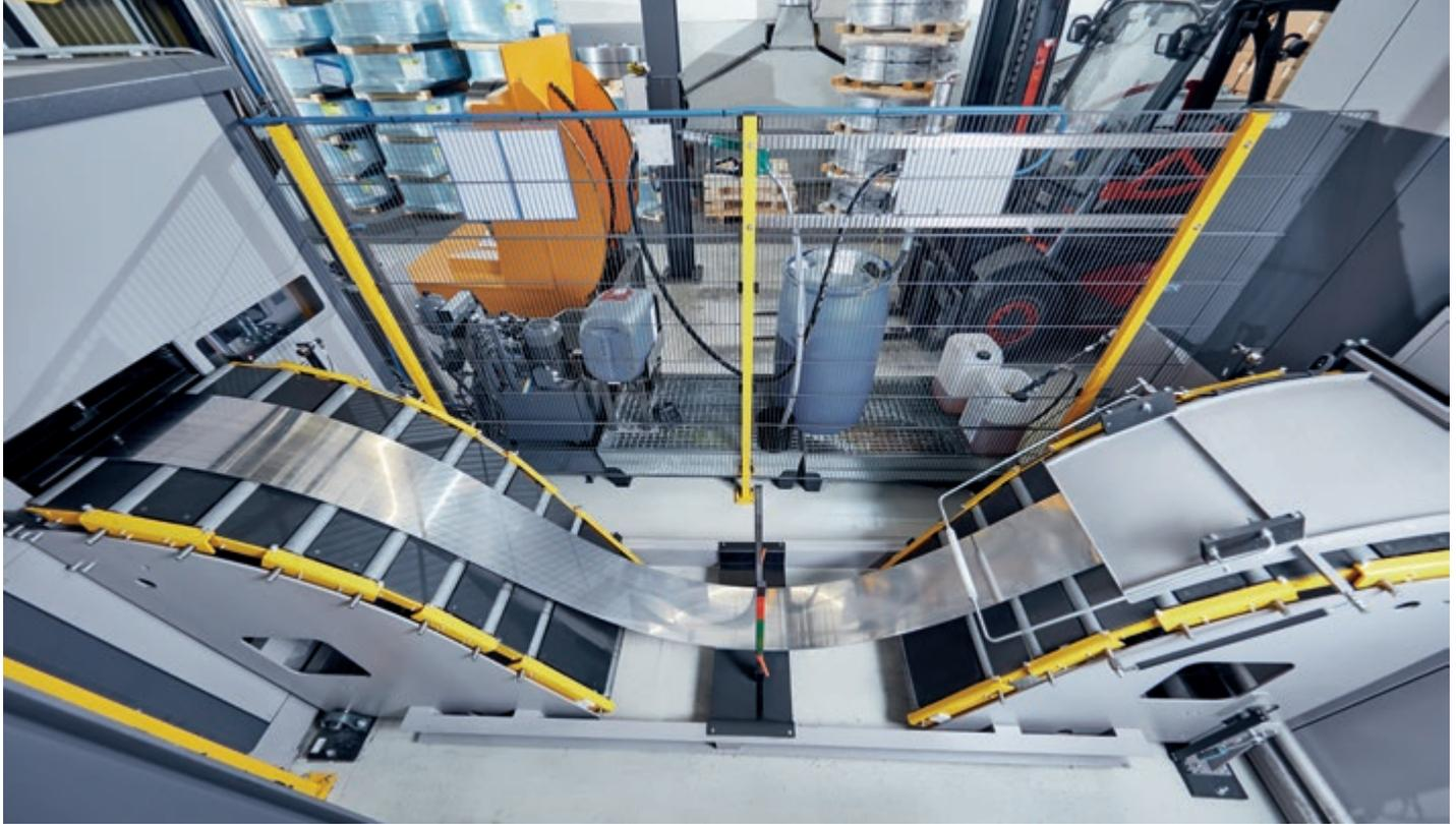
Strip transfer to the downstream high speed punching system. The strip loop between the strip feeding line and the stamping system is designed as a strip transfer table. It ensures a flexible and constant strip supply to the stamping machine.
