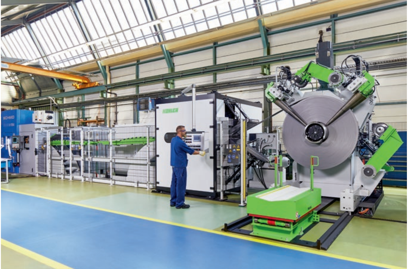
The strip feeding line consists of a stationary coil loading chair, a single decoiler, a 21-roller leveler, and a strip transfer bridge to the downstream press – all adapted to meet the customer's needs.
