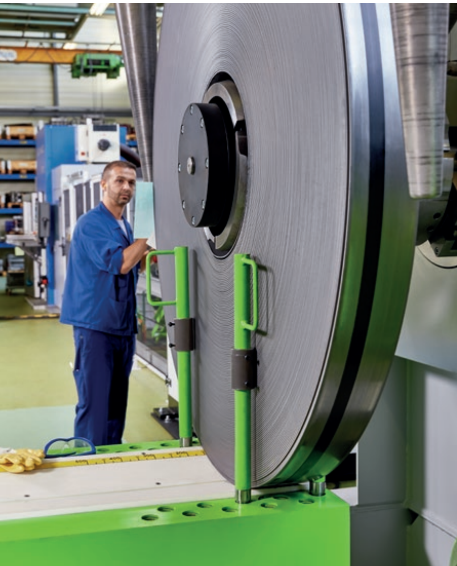
The single decoiler accepts coils of up to 2,000 mm in diameter and 7,000 kg in weight. The stationary coil loading chair can be hydraulically adjusted in height.
