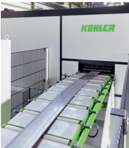
Flexible strip transfer bridge: the strip guidance can be moved into a horizontal position thus creating a strip transfer table.
