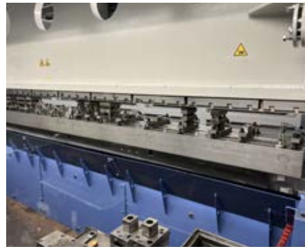
The stroke rate of the stamping machine can be increased to up to 60 strokes at maximum length.
