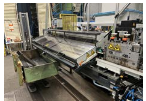
The incoming parts are stopped by the braking system and slide down a chute into the parts container.
