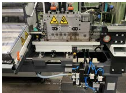
A leveler with 13 leveling rollers produces optimum leveling results after stamping.
