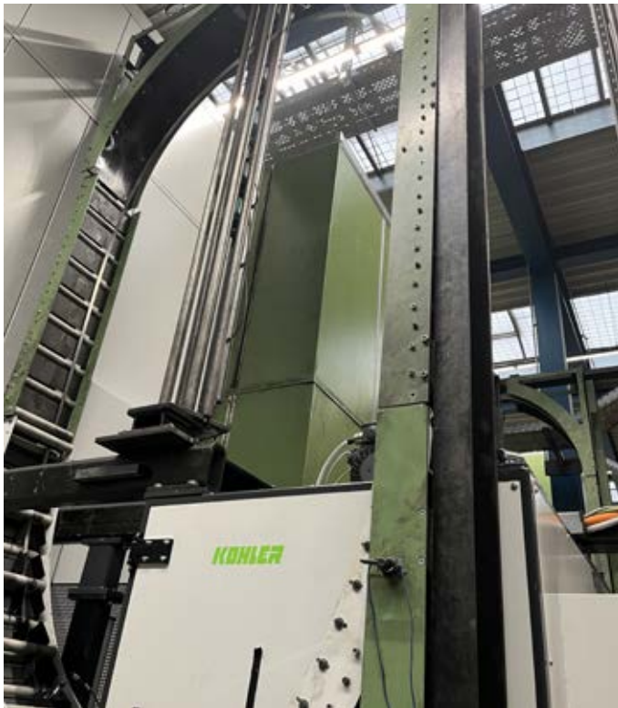
The integration of the loop controller for loop guidance saves space and means less foundation work.
