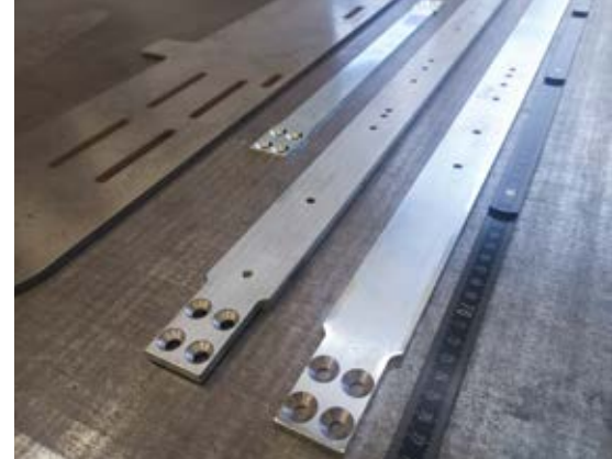
The longitudinal and transverse struts as well as the base panels of the frame are leveled before assembly, in order to satisfy the high requirements for levelness and precision, and to eliminate tension in the material. Photo: German institute for the research and development of sports equipment (FES)
